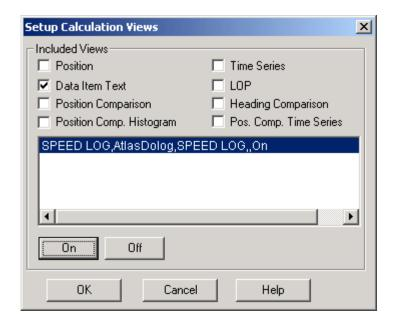
Select (check) the Data Item Text option. Next, highlight the Speed Log data item and click the On button. Exit this window with OK and the speed log data, as well as the Alignment Monitoring data can be viewed in the Calculations window as seen below.
