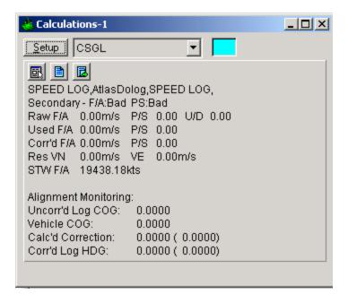
The calculated correction (Calc'd Correction) can be viewed in this window. This correction value can be entered in the Alignment Correction tab.
